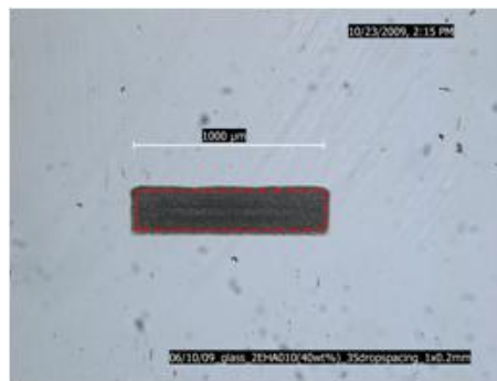
Figure 2: Optical microscopy image of the printing result. The original design is a 1\text{mm} \times 0.2\text{mm} rectangle, represented as the dashed contour.
