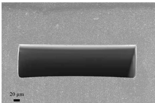
Figure 3: A bonded Viton-Viton channel.
