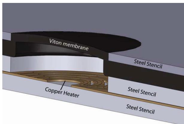
Figure 1: A cross-sectional sketch of the paraffin actuator. The thickness of the stainless steel stencils were 200  $\mu\text{m}$  (lower stencils) and 100  $\mu\text{m}$  (top stencil). To deflect the membrane the paraffin was melted using the heater.
