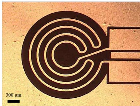
Figure 4: A micrograph of a thin film gold heater patterned on Viton sheet.
