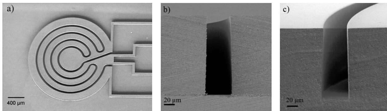
Figure 2: a) An imprint in Viton, b) a close up of its SU-8 template and c) an imprint in Viton at a similar position to that of the template.
