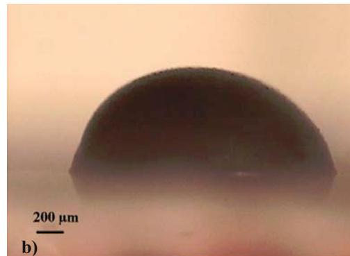
Figure 5: a) Actuator deflection against applied pressure b) An expanded Viton membrane near its rupture limit, actuated by an external pump.
