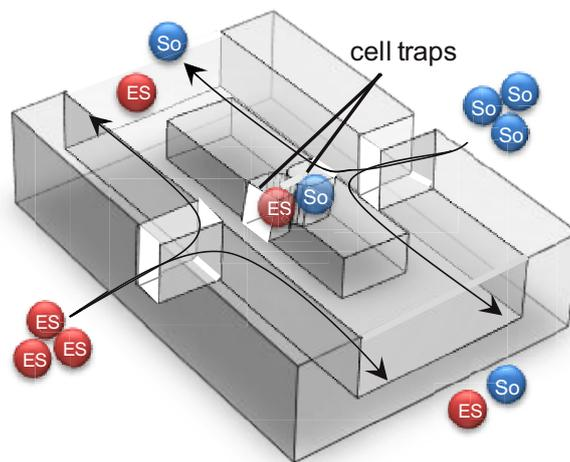
Figure 2. Schematic illustration of cell pairing through microslit in a microchannel.
