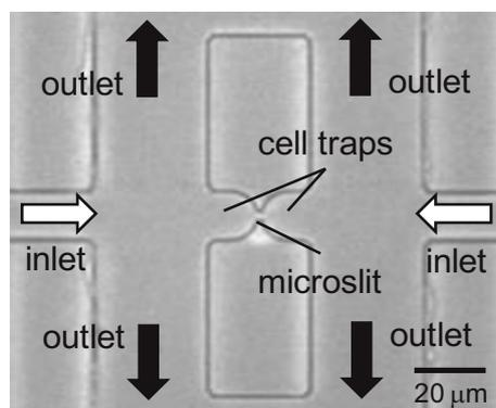
Figure 3. Photo of a microslit and cell traps in the microchannel. Channel depth: 13  $\mu\text{m}$ .
