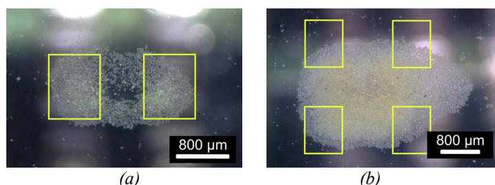
Figure 4: Formation of different patterns and amount of precipitation in DC-704 after approximately 15 minutes by: (a) 2 heaters; (b) 4 heaters. Each heater is supplied with 0.6 W. The liquid is not removed. The yellow rectangles identify the original location of the suspended heaters before they are raised.
