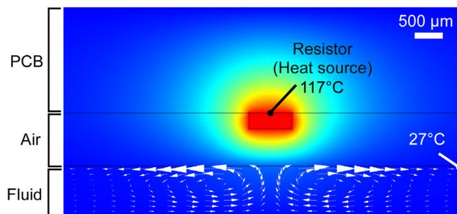
Figure 1: Simulation result showing temperature distribution profile and generated Marangoni flow cells.
