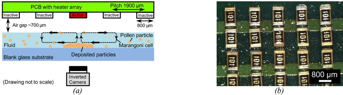
Figure 2: (a) Schematic diagram of experimental setup (side view). (b) Top view of part of the 16 x 8 heater array.
