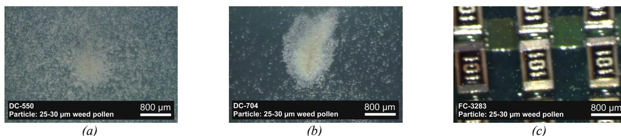
Figure 5: Particle precipitation in three different fluids. (a) Precipitation in DC-550. Particle collection is limited to a small area below the heater. (b) Precipitation in DC-704. More particles are collected from a larger area. (c) No precipitation occurs in FC-3283. The suspended heater is not raised before taking the image.
