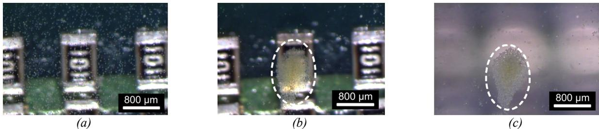
Figure 3: Precipitation in DC-704. (a) Initial random distribution of particles immersed throughout the liquid with approximate concentration of 3-5 particles per  $5 \times 10^6 \mu\text{m}^3$ . (b) Particle precipitation after 4 minutes. (c) Particle precipitation after 12 minutes. Before taking the image, the suspended heater is raised but the liquid is not removed.
