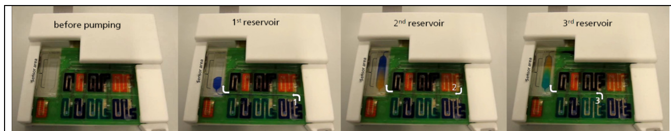
Fig. 2: Pumping process: Emptying of the first three reservoirs by the integrated micropumps. The progress of pumping can clearly be seen by the different colors in the sensor region on the left side. Please note that there is no additional interface to the cartridge than electrical contacts.
