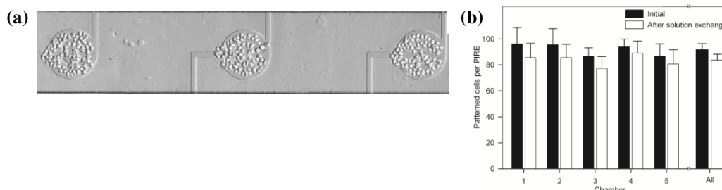
Figure 4. Dielectrophoretic cell patterning (DCP). (a) Patterned cells on a 1 \times 3 collagen-coated PIRE array. (b) Cell count of a PIRE.
