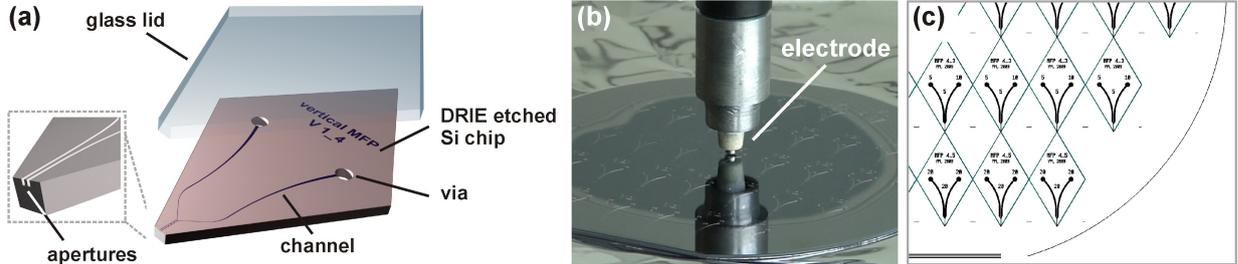
Figure 2: Fabrication of vertical MFP heads. (a) A Si chip comprising channels and vias is closed with a glass lid using anodic bonding. The side of the chip where the channels converge, is cut and polished to define the apertures. (b) Snapshot of the anodic bonding step. (c) Wafer layout showing the dicing lines for easy chip separation.
