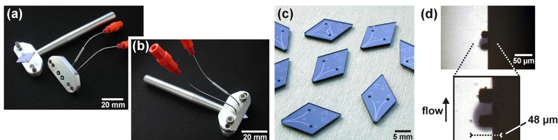
Figure 4. Testing of vertical MFP heads. (a, b) Photographs of a vertical MFP head mounted in a custom made holder comprising connectors for tubes from the pumps. Two rubber O-rings ensure proper sealing. (c) Five different channel/aperture designs were fabricated with channels depths of 10  $\mu\text{m}$  and 20  $\mu\text{m}$ . (d) Micrograph of an operational vertical MFP head, showing the flow confinement using colored water as processing solution and water as immersion liquid.
