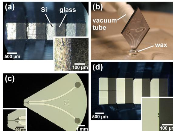
Figure 3: Polishing procedure for vertical MFP heads. (a) Micrographs of unpolished MFP heads clamped into a custom-made holder for lapping and polishing. (b, c) Vacuum assisted filling of the channels with molten wax (140 °C) to protect the channels from debris entering during lapping and polishing. (d) Micrographs of MFP heads after the polishing procedure yielded the well defined apertures.
