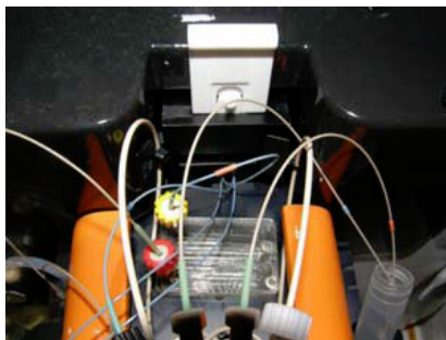
Figure 2: Integration of sample preparation cartridge on to a SPR Navi 200 device
