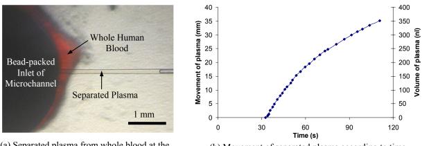
(a) Separated plasma from whole blood at the bead-packed inlet of microchannel
