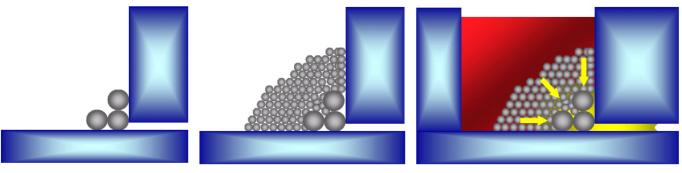
(a) Blocking inlet by packing large beads
