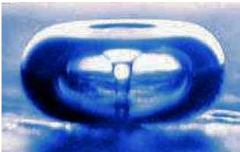
Figure 3 Collapsing cavitation bubble (from [10]).
