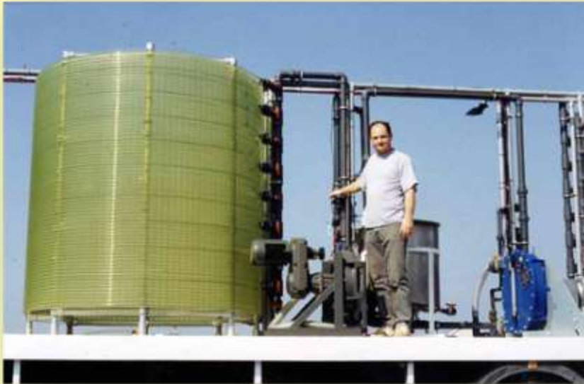
2 stage pilot PBR system (2 x 500 L), with FEP tubing for UV induced secondary metabolite production. Sines, Portugal. Steve Skill (1993)
