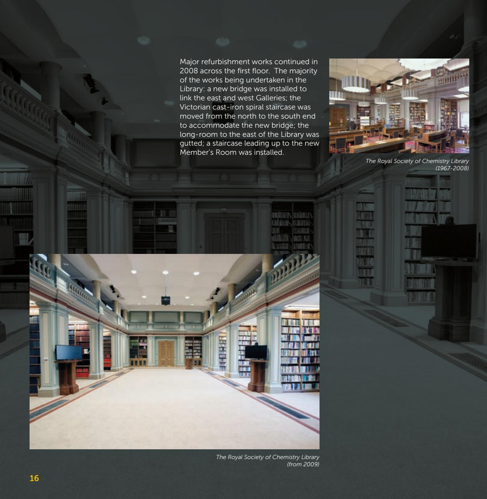
Major refurbishment works continued in 2008 across the first floor. The majority of the works being undertaken in the Library: a new bridge was installed to link the east and west Galleries; the Victorian cast-iron spiral staircase was moved from the north to the south end to accommodate the new bridge; the long-room to the east of the Library was gutted; a staircase leading up to the new Member's Room was installed.
