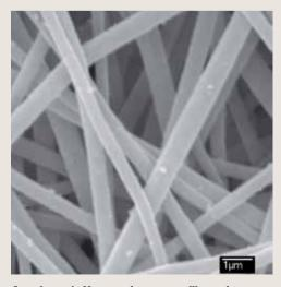
Arteriocyte's Nanex polymer nanofibre substrate for rapid stem cell culturing
