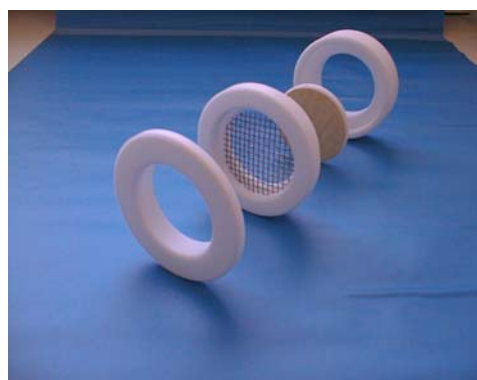
Chemcatcher – exploded view
