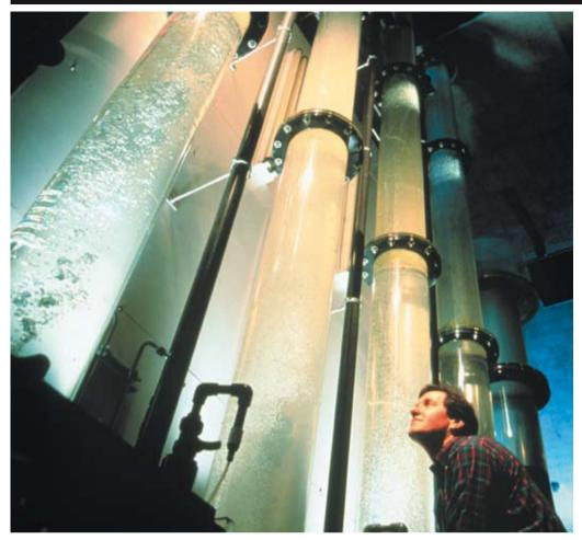
destabilise colloidal particles); flocculation (agitating coagulated water to promote the aggregation of suspended materials); and sedimentation (where flocculated water is stilled to promote settling of suspended solids and floccules). The water is then usually chlorinated.
