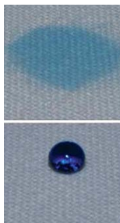
Water spreads in the plainweave polyester fabric and forms a droplet on the TiO 2 -silica coated polyester fabric
