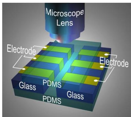
Figure 1. Schematic diagram of the microfluidic device integrated with sidewall electrodes in the channel. The sidewall electrodes are defined onto the top and the side surfaces of a glass slide by applying a shadow mask with slits during metal evaporation. Two patterned glass slides are placed side by side and sandwiched between two thin layers of solid PDMS.
