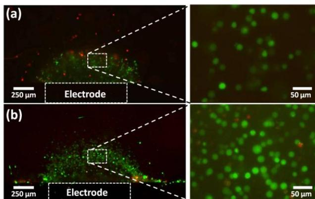
Figure 4. Fluorescent micrographs of NS0 cells entrapped in the electrodeposited calcium alginate gel. (a) before and (b) after culturing (3 days). The two insets show a magnified view of the assembled cells entrapped in the gel before and after culturing.
