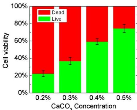
Figure 3.  $\text{CaCO}_3$  concentration dependent viability assessment of assembled NS0 cells in the electrodeposited calcium alginate hydrogel.
