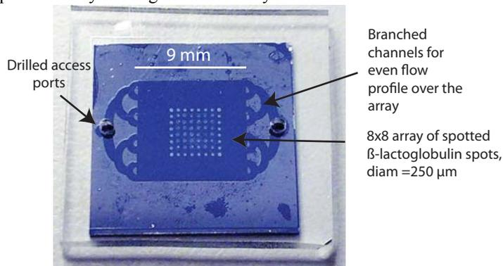
Figure 3: A Biosticker flow cell attached to the protein microarray. The spots are visible through the polymer. To guarantee an even flow profile over the spots, branched inlet and outlet channels are used.
