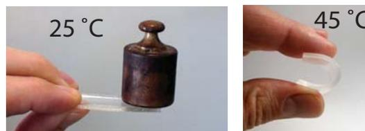
Figure 1: The Biosticker material is hard and stiff at room-temperature but when heated to 45 °C it becomes rubbery.
