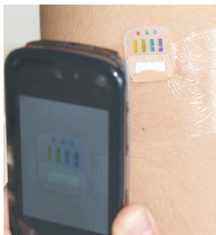
Figure 2: Wearable micro-fluidic device located on the arm using a high adhesive transparent sweat patch. The camera of a mobile is using to take pictures of the sensing area of the device. The mobile application will be used for real time pH monitoring of sweat during exercise.
