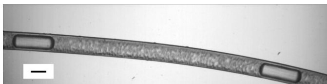
Figure 4. Polyethylene tubing containing droplet libraries separated with air bubbles. Scale bar is 1 mm
