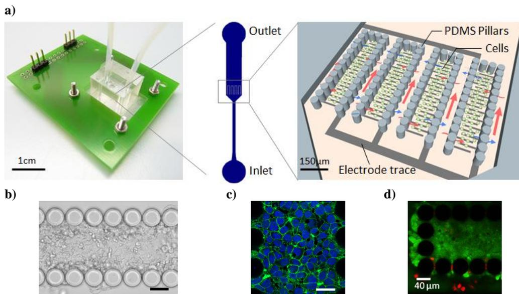
Figure 2: Microfluidic cell culture. a) Microfluidic device with electrical interface (left), perfusion channel design (middle), cell culture area involving PDMS pillars for cell immobilization and electrodes (right), b) Brightfield image of cells within a filter structure (without electrodes), c) Close cell-cell contacts are visualized through occludin staining (green=Cy-2, blue=DAPI), d) Life/dead staining (green=fluoresceine-diacetate; red=propidium-iodide). (bars=40 μm)
