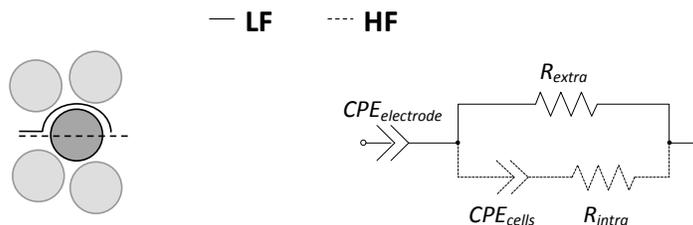
Figure 1: Left: Schematic of current pathway at low and high frequency, Right: Equivalent circuit of electrode-cell population model
