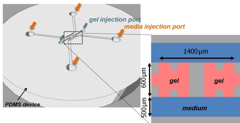
Figure 1: Microfluidic platform
