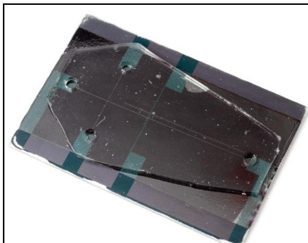
Figure 1: Photograph of a completely polymer microchip with integrated conducting polymer high voltage electrodes and detection electrodes.
