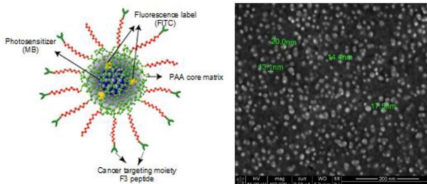
Figure 2. (a) Schematic of the functionalized nanoparticles. (b) SEM images of the MB-loaded fluorescent nanoparticles.
