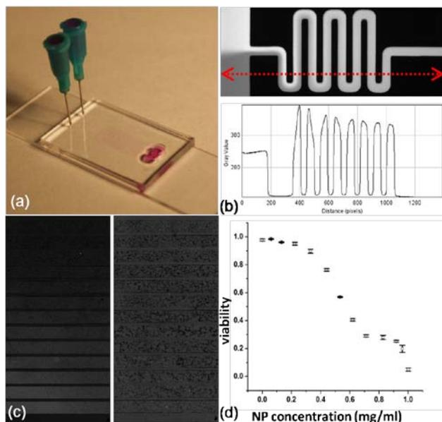
Figure 4. (a) Gravity flow setup, (b) Fluorescent image of NP mixing in the chip, (c) NP incubation with a gradient (left) and after being washed away (right), (d) C6 cell viability as a function of different NP concentration.
