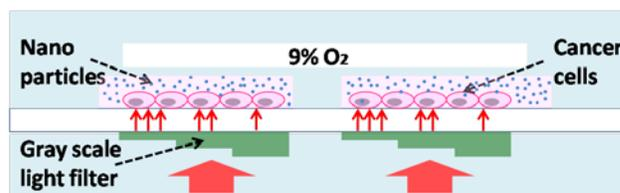
Figure 1. Cross-section view of a typical microfluidic chip we used in this work for PDT assays.
