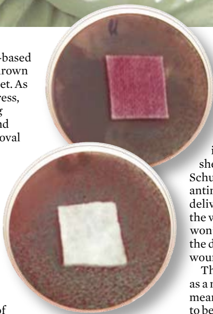
Quick-Med, US, has developed a polymeric antibacterial wound dressing – Nimbus. The untreated dressing (top) is overridden with bacteria while none survive on the Nimbus-treated dressing
