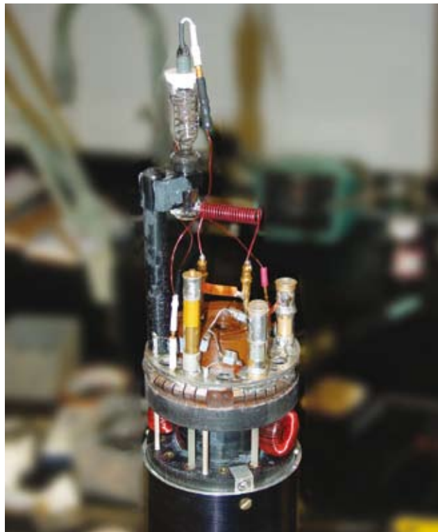
Value-added NMR: compared to conventional NMR probes the in situ electrochemical NMR probe (above) developed by Tong and his team at Georgetown has to accommodate an electrochemical cell, part of which is inside the NMR detection coil
