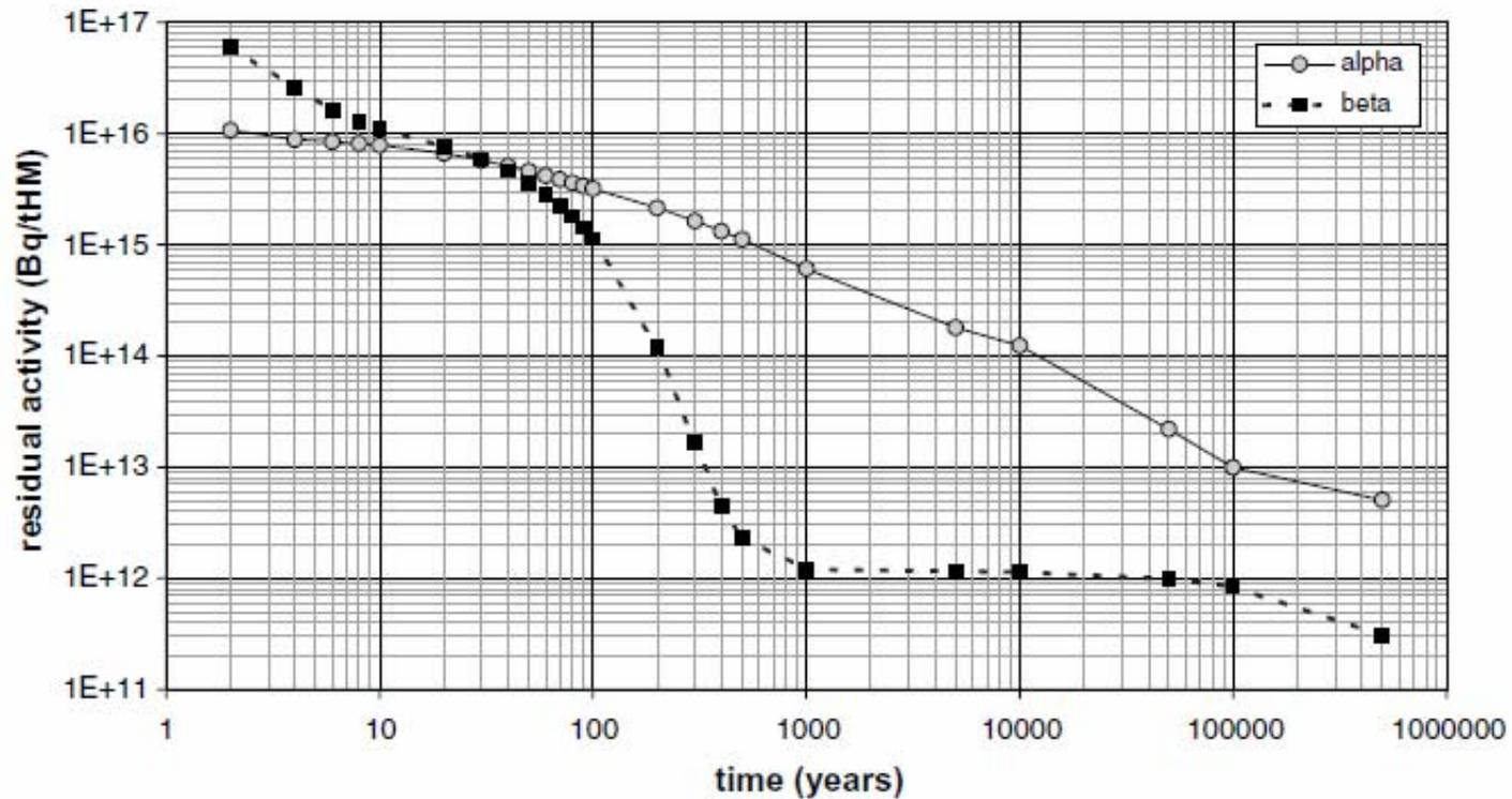
Fig. 1. Evolution of  $\alpha$ ,  $\beta$  and  $\gamma$  radiations as a function of time for a  $55 \text{ GWd t}^{-1}$  UOX fuel. Data are calculated from the CESAR isotopic evolution code [35].
