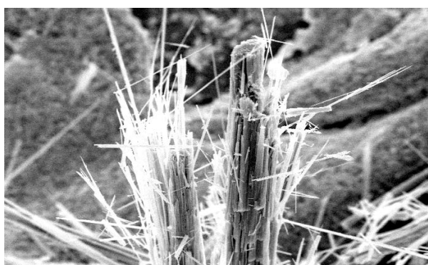
Figure 1. Asbestos tremolite fibres under scanning electron microscopy
