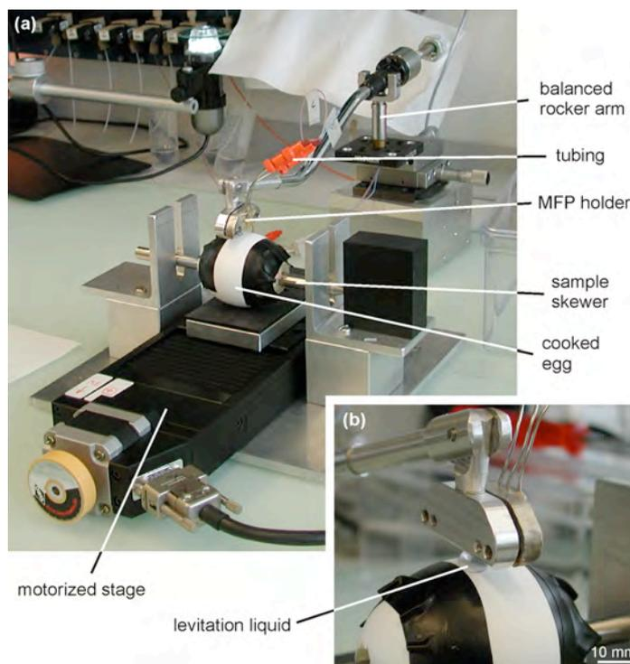
The vMFP head was mounted in a custom aluminum holder prior to performing an experiment. The syringe pumps (not shown) were connected to the holder through capillary tubing. O-rings were used to seal the connection between the vias of the vMFP head and the ports in the holder.
