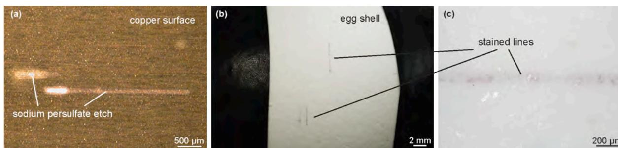
**Figure 3.** Local processing of "challenging" surfaces. (a) A 35- $\mu\text{m}$ -thick Cu surface was locally etched using a confined  $\text{Na}_2\text{S}_2\text{O}_8$  solution (20% w/v). (b) and (c) Lines of 75 to 100  $\mu\text{m}$  width stained with logwood brew on the shell of an egg using the levitating MFP.
