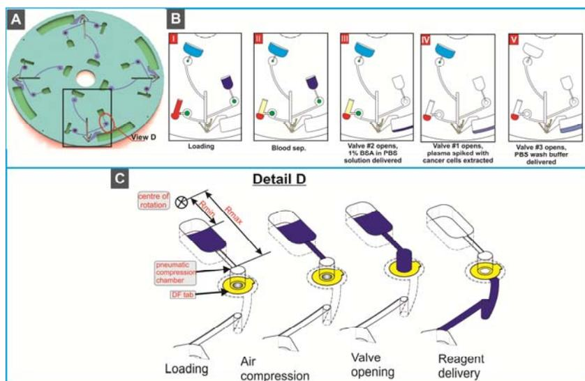
Figure 1 a) 3D illustration of the DF-based centrifugal platform b) schematic illustration of the multi-step IA c) Step-by-step demonstration of the DF valve actuation by rotation of the disc.
