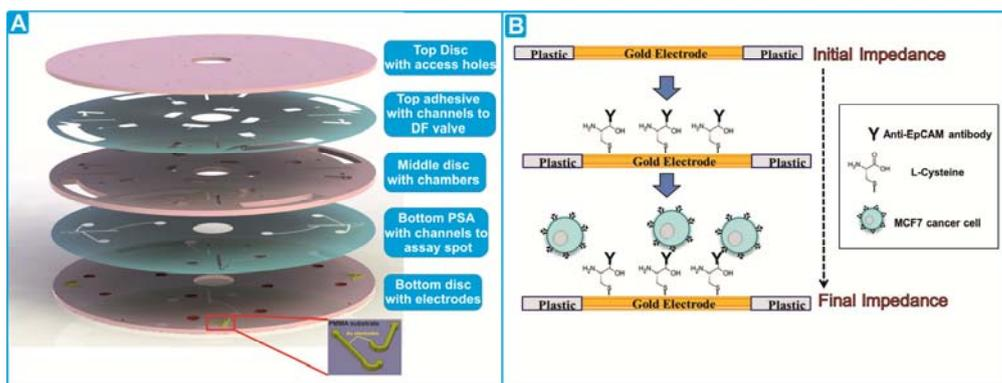
Figure 2: a) 5-layer disc assembly. 2 adhesive layers are interspersed between 3 plastic substrates. b) Schematic illustration of the surface chemistry, Ab immobilization and cell capture. Initial impedance measurements are carried out before Ab immobilization and after cell capture.
