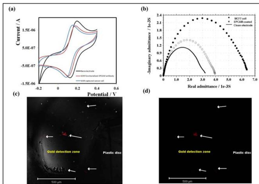
Figure 4: a) Cyclic voltammery showing the different curves for the bare electrode, with Ab and with cells b) Corresponding EIS measurements c-d) fluorescence images of the captured cells on the Au electrodes. Capture and detection of the cancer cells was carried out off-chip.
