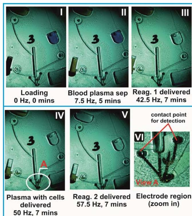
Figure 3: I-V) Frame sequence of the multi-step IA showing blood separation and sequential reagent release. In order to enhance contrast, 1% v/v food dye was added to PBS buffer, and pre-loaded in the reagent chambers. VI) View of the electrode region and contact point for electrochemical detection.
