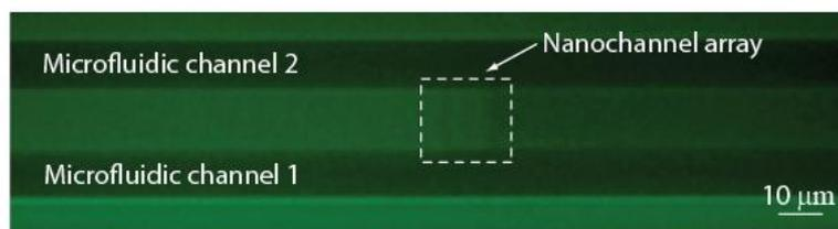
Figure 3. Nanochannel bridge. The nanochannels embedded between two open microchannels. This preliminary test showed that a nanochannel array could be integrated into the pre-built microfluidic-system.
