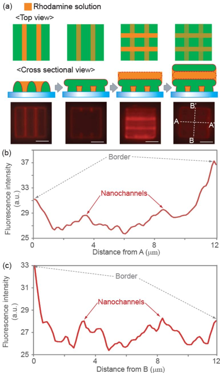
Figure 4. Vertical array of nanochannels. (a) Vertical array of nanochannels fabricated by laser-writing process in Fig. 2. The dye solution could flow into the nanochannels. Scale bars indicate 5 μm. Fluorescence intensity along line (b) AA' and (c) BB'. 4 nanochannels in the vertical array could flow the dye solution. The border of the structures glowed due to dye absorption.
