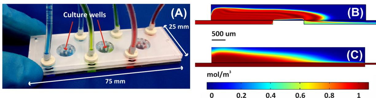
Figure 2: Picture of the fabricated device during the fluidic test (A), simulated concentration profile inside the culture chamber for the design implementing convection through the membrane after 2 sec (B) and for design enabling diffusive delivery of drug after 60 seconds (C).
