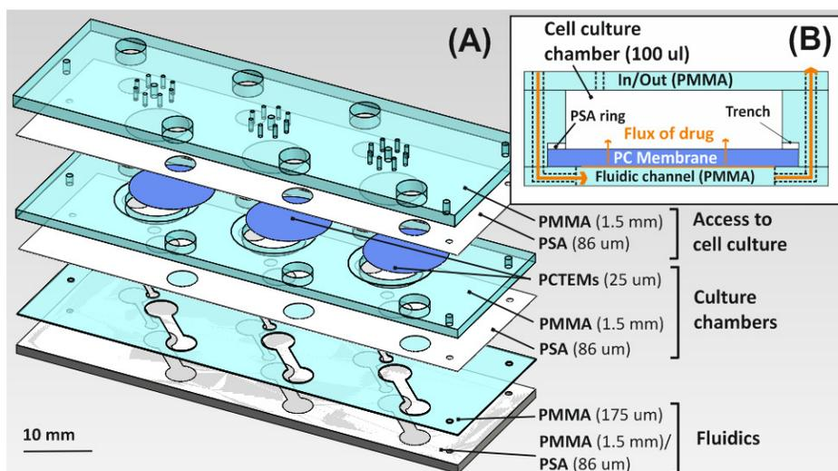
Figure 1: 3D schematic of the device assembly (A) and cross sectional view (B). The device consists of three main compartments: (i) fluidic structures defined in the bottom PMMA/PSA layer, (ii) PMMA culture chambers with integrated GE Whatman® polycarbonate track-etched membranes installed on PSA rings and (iii) a PMMA cap with inlets to introduce cell culture and gaps to supply sufficient aeration of cells.
