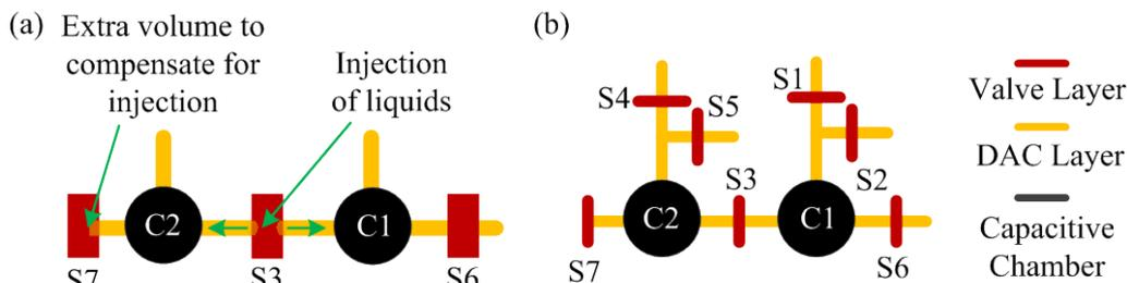
Figure 3: Improved design for volume injection correction. (a) When S3 closes, some volume of incompressible fluid is displaced into C2, increasing output pressure. S7 opens when S3 closes to accommodate volume injection. (b) The final improved design is insensitive to small  $x y$  alignment errors and corrects for volume injection.
