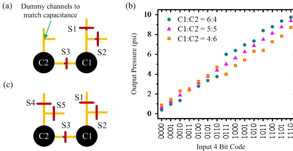
Figure 2: Alignment error insensitive design using dummy valves. (a) Alignment errors in x and y result in mismatched capacitances (purple) when fixed dummy channels are used to mirror design geometry (green arrow). (b) Simulation show that mismatched capacitors result in nonlinearity in output transfer function of the microfluidic DAC. (c) Adding dummy valves S4 and S5 reduces possible mismatch between C1 and C2. Y alignment errors now have no effect on capacitive mismatch.
