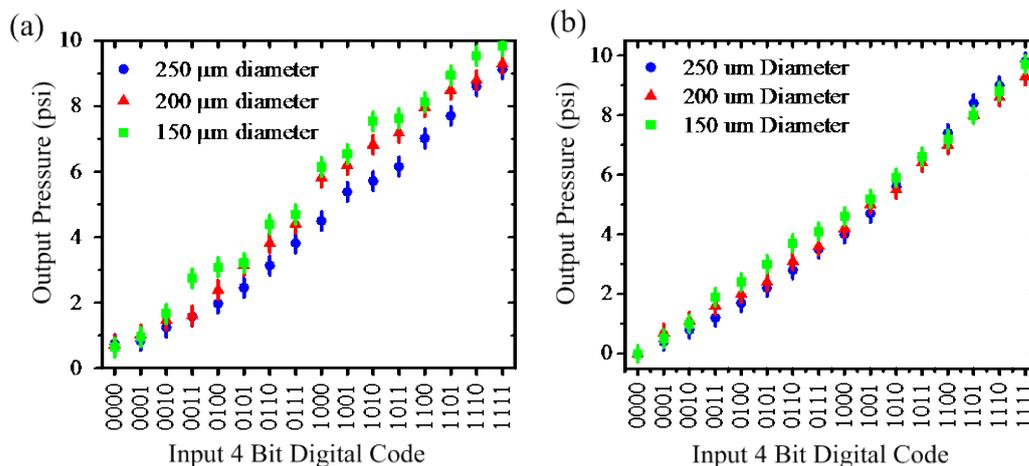
Figure 4: Comparison of the microfluidic DAC performance before (a) and after (b) implementing the new design demonstrates significant improvements in output linearity. In fact, with better matched capacitors and correction for volume injection, we see that the DAC output is independent of membrane diameters.
