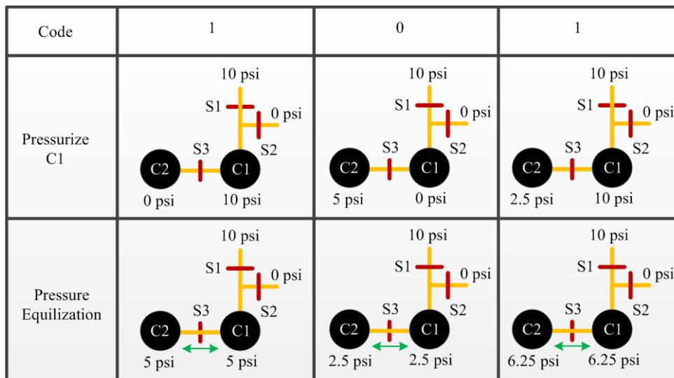
Figure 1: Microfluidic serial pressure DAC functionality depends on two operations per cycle. During each cycle, C1 is pressurized to 10 psi or 0 psi depending on the digital code. Then, switch S3 is used to perform pressure equalization, where pressures in C1 and C2 are set equal. This figure demonstrates steps required to generate 6.25 psi with a 10 psi supply and a 3 bit digital code of 5 (or 101 in binary). The code is processed from the most significant bit to the least significant bit.
