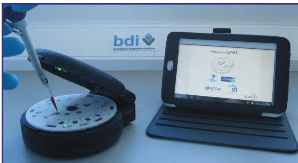
Figure 1. Image showing loading of blood sample and assay reagents on the portable LoaD system interfacing with an Android tablet. A customized program controls the time modulated spin speed of the disc as well as the wireless acquisition of real-time data. On completion of the full assay protocol, the LED-based system is then used for colorimetric detection of the assay panel.
