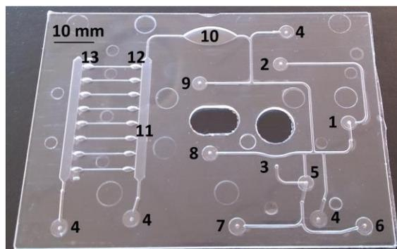
Figure 2: Microfluidic chip. (1) Sample inlet valve; (2) lysis buffer inlet valve; (3) extraction chamber transfer point; (4) waste outlet valves; (5) valve; (6) wash buffer 1 inlet valve; (7) wash buffer 2 inlet valve; (8) elution buffer inlet valve; (9) reagents inlet valve; (10) mixing chamber; (11) broad channel; (12) pre-NASBA chambers; (13) NASBA chambers.
