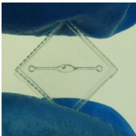
Figure 3: Freeze-dried sphere inside a 2  $\mu\text{l}$  COP chamber bonded with PCR film, developed at IK4-Ikerlan S.Coop, supplied by MicroLIQUID., Spain.
