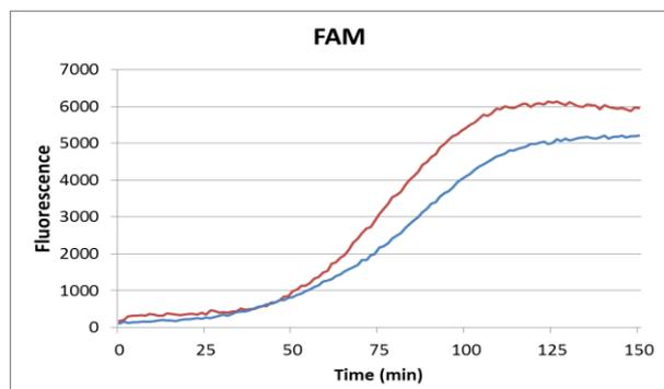
Figure 5: Conventional NASBA run on bacterial nucleic acids extracted in the POCNAD cassette (red line) and by conventional extraction method (control, blue line).
