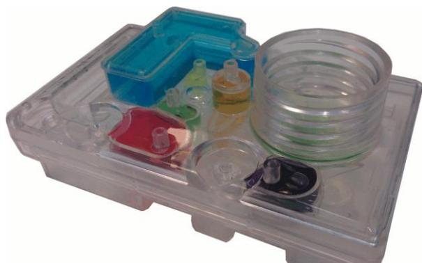
Figure 1: POCNAD cartridge. Reagents are stored in the top part: lysis buffer (blue); NASBA reagents (yellow); elution buffer (green); extraction chamber with silica beads (orange); and wash buffers (purple and pink).
