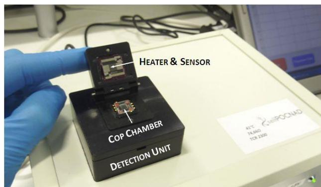
Figure 4: The NASBA reader for the testers. The device performs a customized thermal cycling and double channel fluorescence reading, developed at IK4-Ikerlan S. Coop.
