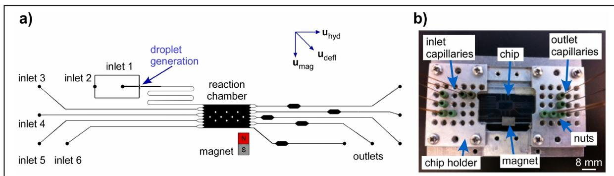
Figure 2: (a) Chip design for droplet generation via flow focusing and deflection through a reaction chamber. The droplet generation region was etched to a depth of  $20\ \mu\text{m}$  in one glass layer, and the remainder of the design was etched to  $100\ \mu\text{m}$  in a second glass layer. (b) Photograph of the setup showing the glass chip in its holder with inlet and outlet capillaries, and a permanent magnet.
