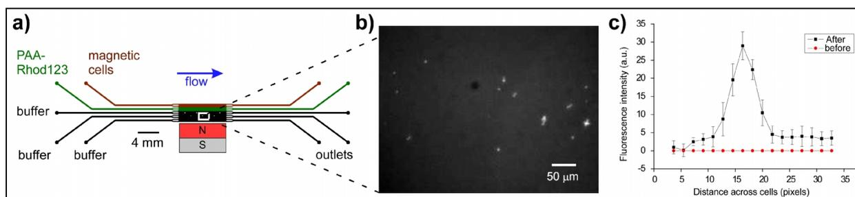
Figure 5: Deflection of PVP-coated magnetic yeast cells through negatively-charged PAA-Rhod123. (a) Schematic of chip design and flow streams. (b) Photograph of fluorescent yeast cells after leaving the PAA-Rhod123 stream. (c) Plot of fluorescence intensity across the cells before and after passing through the PAA-Rhod123 stream. Cells exhibited no fluorescence prior to the reagent stream.
