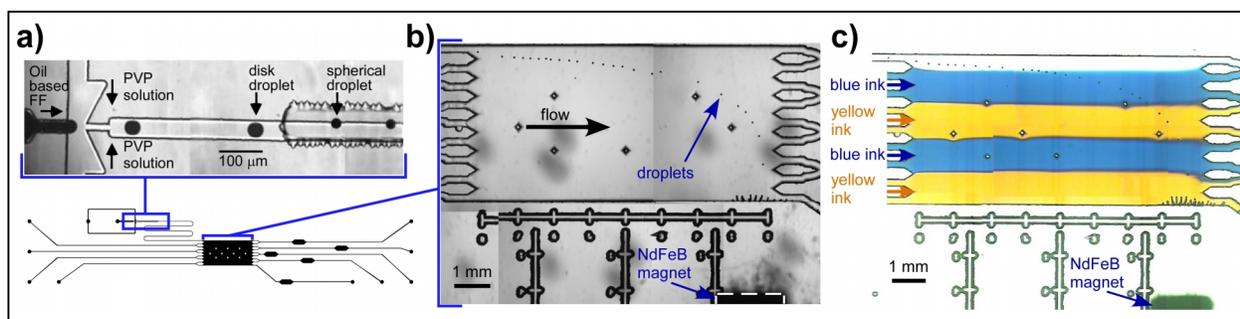
Figure 3: (a) Two-layered device for generation of small, spherical FF droplets. (b) Deflection of droplets across chamber (flow in chamber  $1.2\ \text{mm s}^{-1}$ , magnetic force 320 pN). (c) Deflection of droplets through multiple laminar flow streams of aqueous inks.
