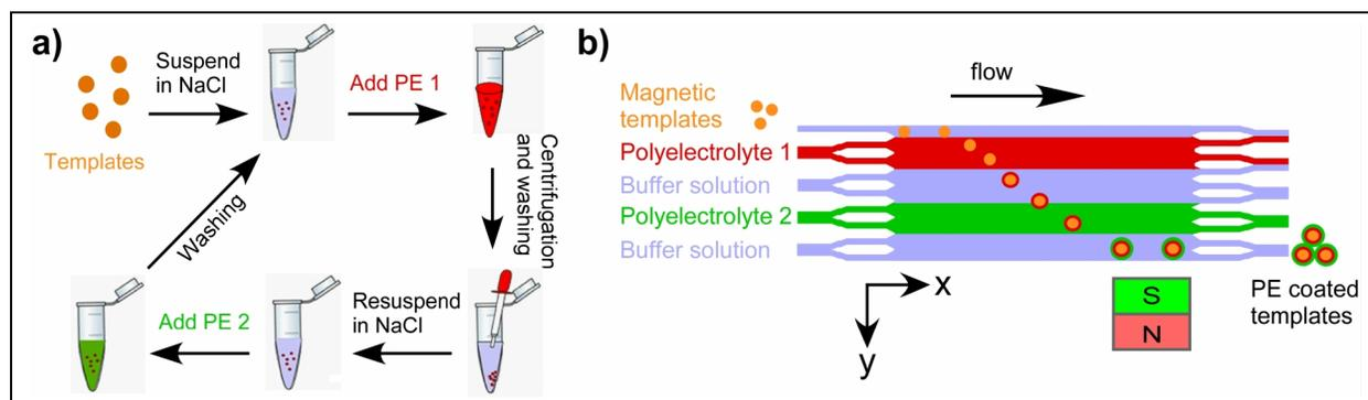
Figure 1: (a) Conventional LbL deposition of polyelectrolytes (PE) using tubes and centrifugation. (b) Concept of continuous flow layer deposition on magnetic templates in a microfluidic device.
