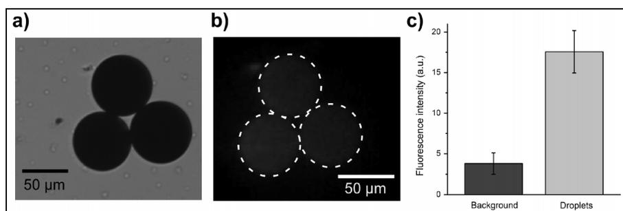
Figure 4: PVP-coated ferrofluid droplets after passing through the PAA-Rhod123 stream: (a) microscope photograph, (b) fluorescence image, (c) fluorescence increase against background.
