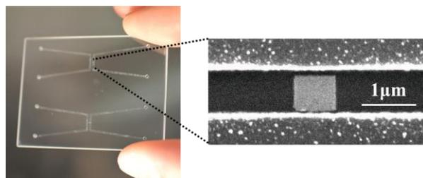
Figure 2: The picture of SNC chip (a), and SEM images (b) of the gold nanopatterns in nanochannel: 800 nm wide and 300 nm deep.
