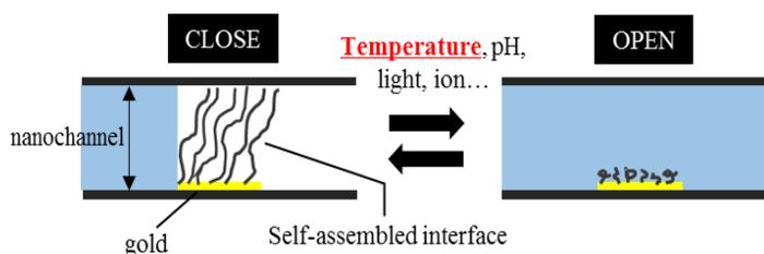
Figure 1: The concept of smart nanofluidic control (SNC).
