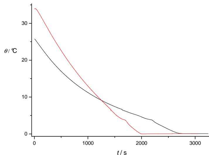
**Fig. 1.** Cooling and freezing of deionised water ( $V = 30$  ml) at  $\approx 25$  and  $35$  °C in a glass beaker with no cover, without mixing.
