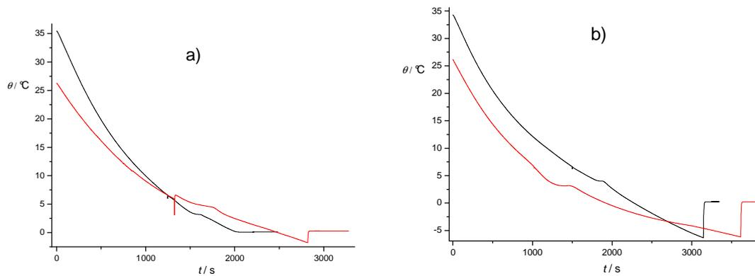
Fig 2. Cooling of 30 ml of deionised water in an icebox with controlled conditions, without mixing.
