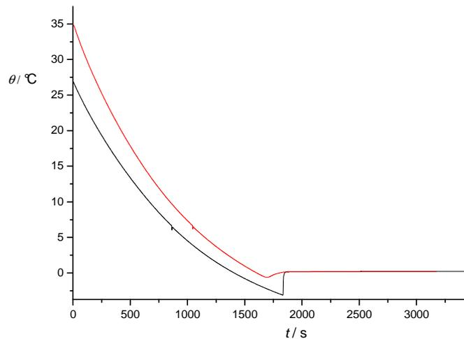
Fig 4. Cooling and freezing of deionised water ( $V = 30$  ml) at  $\approx 25$  and  $35$  °C in a glass beaker with mixing.
