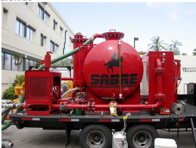
A mobile chlorine dioxide generator used for decontamination
