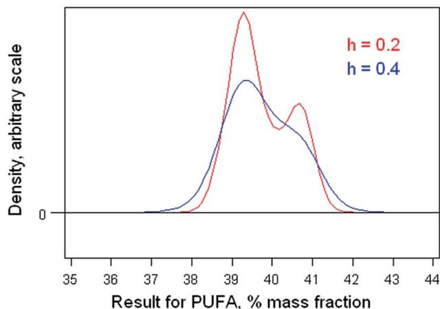
Fig. 4 Kernel densities of results for PUFA with smoothing parameters of 0.2 and 0.4.
