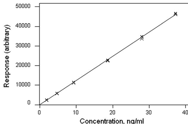
Fig. 1 Calibration data (crosses) and fitted function (line) for aflatoxin M1.
