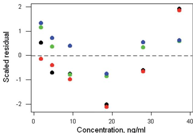
Fig. 2 Aflatoxin M1 calibration: plot of scaled residuals, colour-coded by response set, after weighted linear regression.
