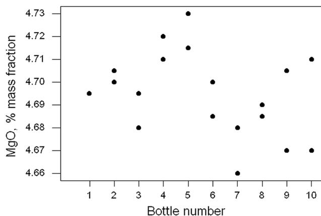
Fig. 5 Homogeneity test: duplicate results (points) for MgO in ten samples of a rock powder. Sample 1 has two coincident results.
