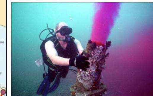
Figure 2&3 Rhodamine dye tests undertaken at the Perth Seawater Desalination Plant (Water Corporation, 2006).
