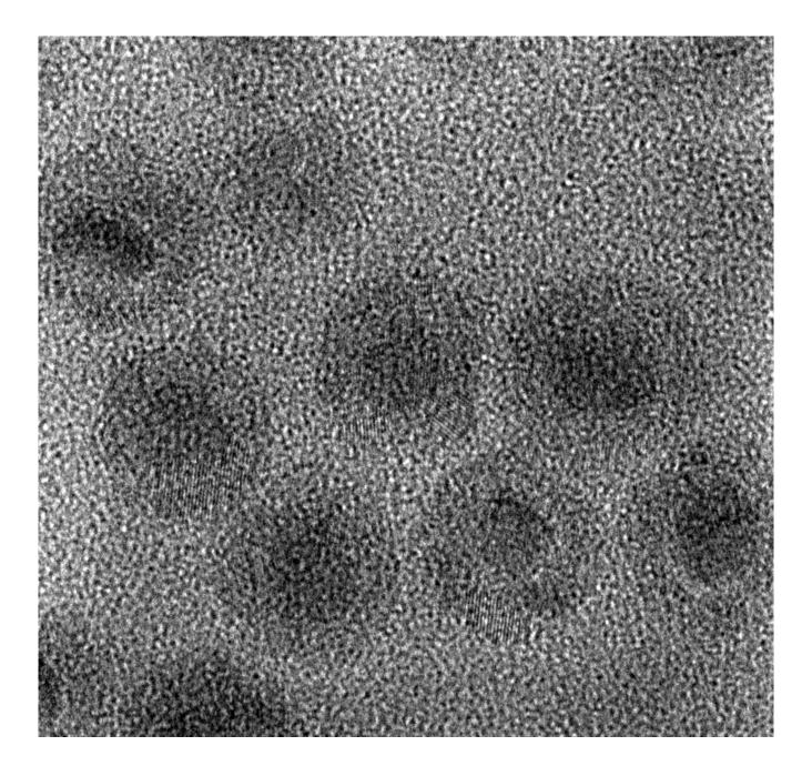
Figure S1c. High-resolution TEM image of  $In_2O_3$ - $In_2S_3$  nanoparticles.
