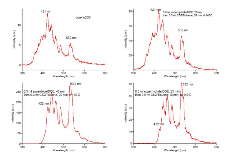
Figure S2. Photoluminescence spectra recorded with various reaction conditions, showing that the reduction step is more important than the sulfidization step for the formation of  $In_2S_3$  shell.
