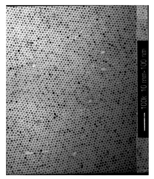
Figure S1a. TEM image of  $In_2O_3$  core nanocrystals.
