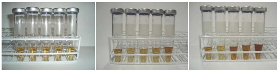
Fig. 2 Dissolution of cellulose in [C_2MIM]Cl under microwave irradiation: a) 6 wt-% of cellulose, 100 °C, power between 60 and 140 W, b) 2 – 10 wt-% of cellulose, 140 °C, 80 W, 30 min, c) 2 – 10 wt-% of cellulose, 160 °C, 80 W, 30 min.
