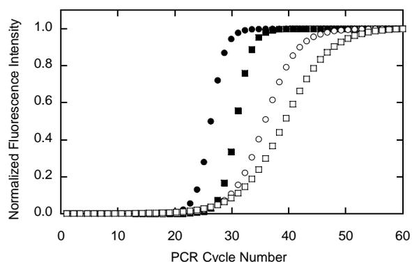
**Fig. S3** On-cartridge real-time PCR. The real-time fluorescence curves of serial diluted ((●) 0-fold, (■) 10-fold, (○)  $10^2$ -fold and (□)  $10^3$ -fold) influenza A, amplified and measured with the custom-built thermal cycler and detection system.
