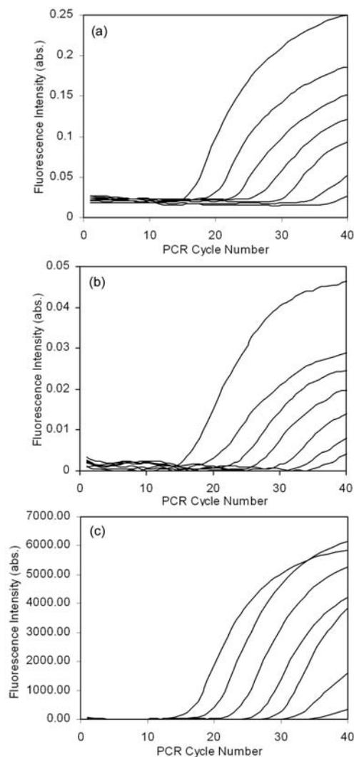
**Fig. S2** On-cartridge real-time PCR. The real-time fluorescence curves of serial diluted ( $1-10^6$  folds) GAPDH cDNA, amplified and measured with (a) the custom-built thermal cycler, (b) the MJ Research Opticon system, and (c) the Bio-Rad CFX96 system. The custom-built thermal cycler utilized LEDs as light source and a PMT for detection, the MJ Research Opticon system employed LEDs plus PMTs, and the Bio-Rad CFX96 system used LEDs and photodiodes.
