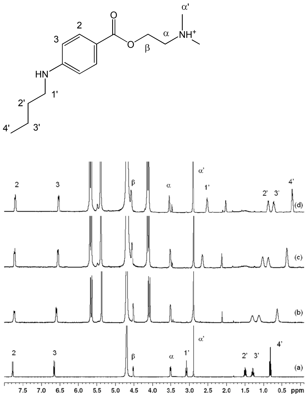
Figure S5. 1 H NMR titration of tetracaine (1.33 mmol dm -3 ) with CB[7] in D 2 O. (a) 0.0 equiv, (b) 0.40 equiv, (c) 0.84 equiv, and (d) 1.29 equiv of CB[7].
