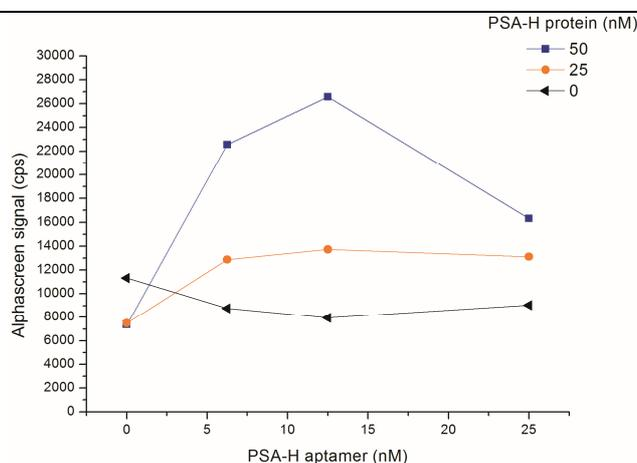
**Figure S3. Saturation assays of streptavidin-coated donor beads.** Various concentrations of biotinylated aptamer were incubated with constant amount of protein in binding buffer. The mixtures were further incubated following the addition of an equal concentration of donor and acceptor beads. The luminescence signal maximum was identified at 12.5 nM biotinylated aptamer indicating the binding capacity of 25  $\mu$ l of donor bead at 20  $\mu$ g/ml concentration.
