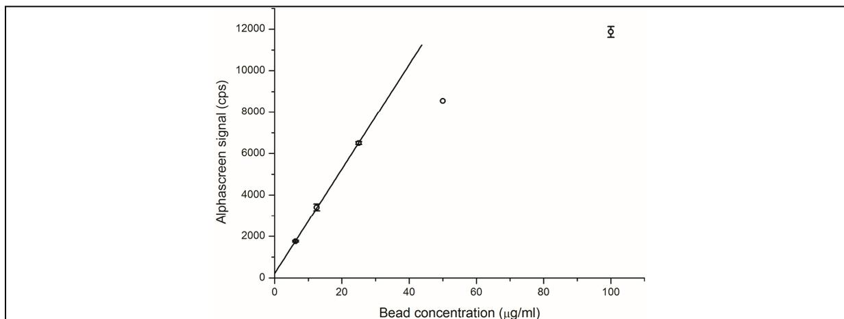
**Figure S4. Correlation between bead concentration and AlphaScreen signal.** Various amounts of beads were incubated with the positive control Biotinylated-6His. The background corrected data (experimental background =  $1443 \pm 302$  cps) indicates that the signal is elevated upon increasing the bead concentration but there is a deviation from linearity at concentrations higher than ca. 25 µg/ml.
