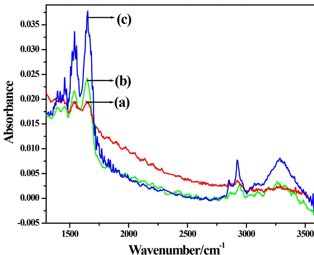
**Supplementary Fig. 1** FT-IR spectra of (a) PDDA, (b) PDDA-SWCNT, and (c) H1N1 antibody immobilized PDDA-SWCNT.
