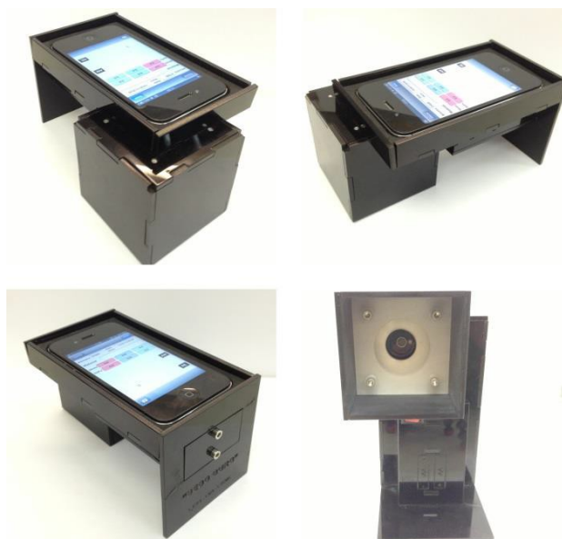
Figure S1: Photographs of different angles of the smartphone support with the smartphone.
