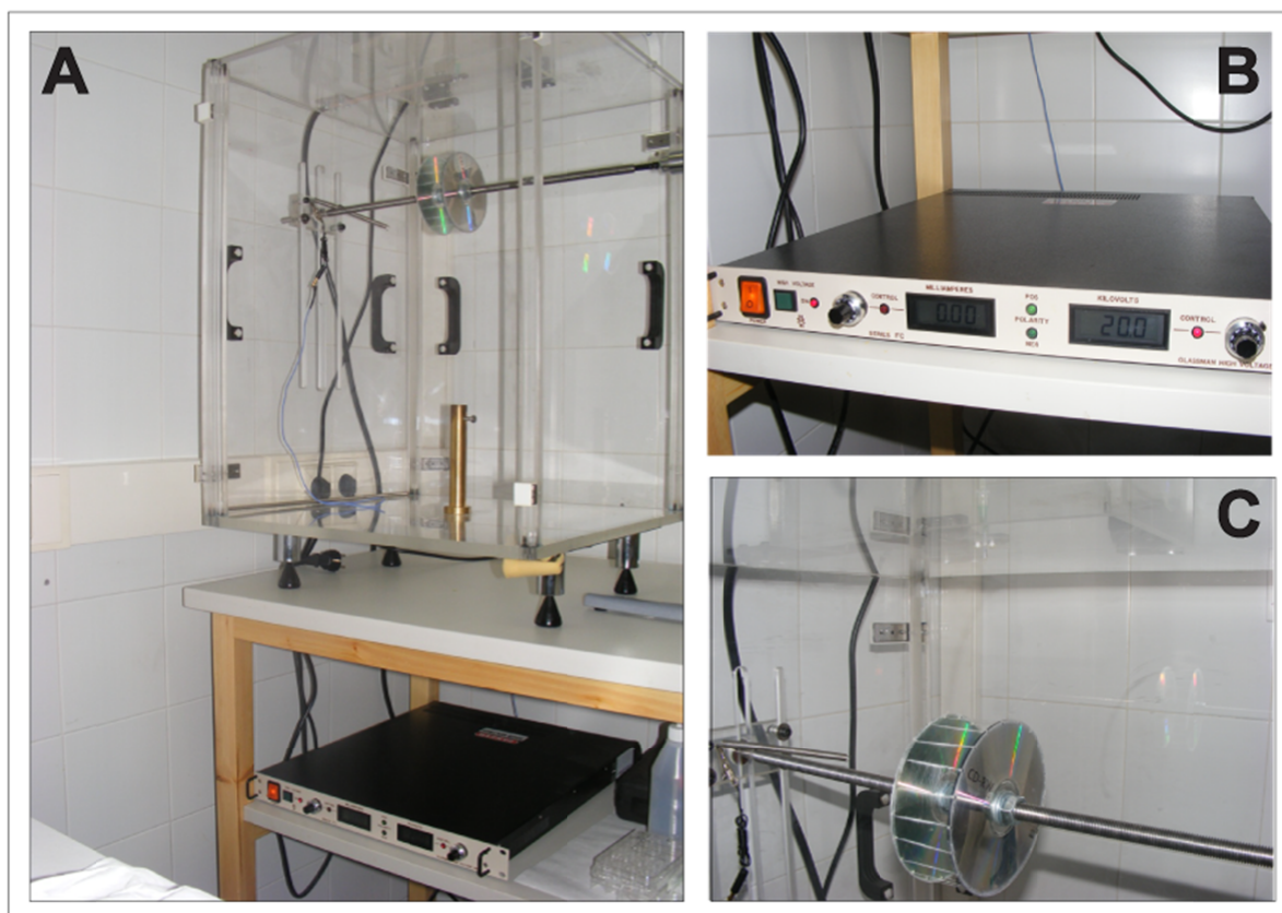
Supplementary Fig. 1: The electrospinning setup developed for fabrication of FBG nanofibers. Overview (A); High voltage supply (B); Rotating drum with parallel metal wires for collection of aligned nanofibers (C).
