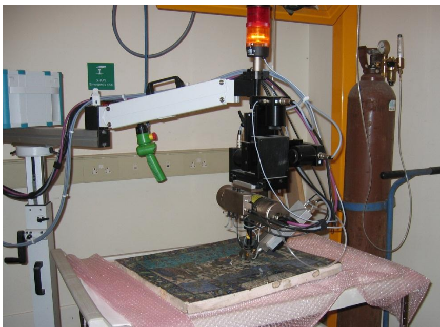
Figure 19.7 Micro-EDXRF set-up (ArtTax) with He purging used for the analyses of the glaze and the body of the tiles 510–1889 and 511–1889 at the Victoria and Albert Museum, London. Tile shown is 510–1889, © I. Reiche, 2006.
